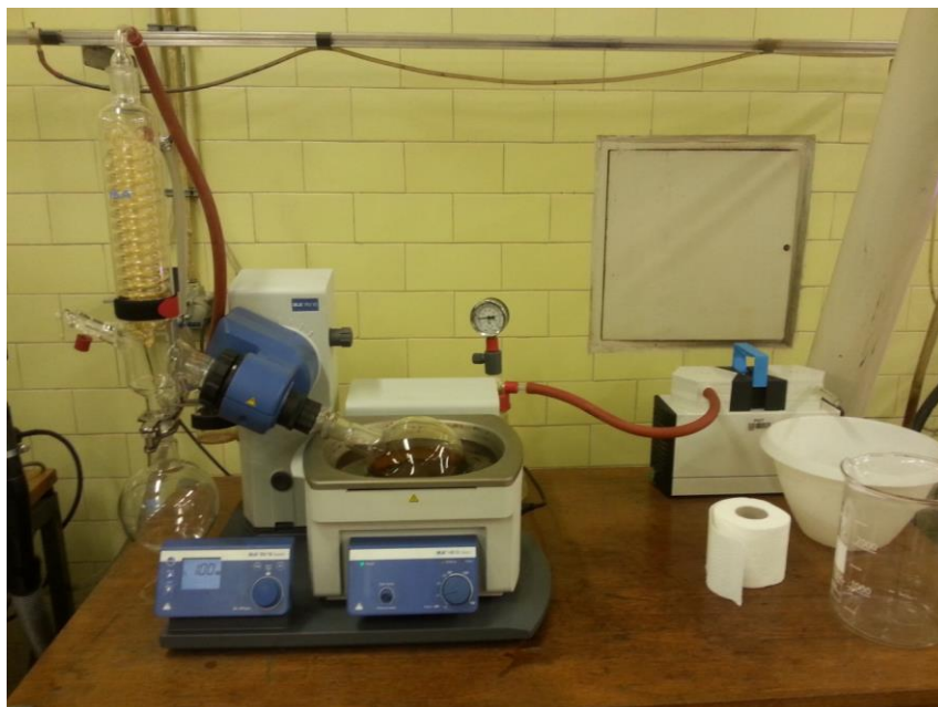
Slika 13. Vakuum isparivač (IKA RV 10, rotary evaporator, basic ) s vakuum pumpom (KNF LAB LABOPORT)
