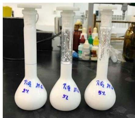
**Slika 3.8.** Priredjene otopine  $\text{TiO}_2$ ,  $w(\text{TiO}_2) = 2 \text{ } \%, 3 \text{ } \%$  i  $5 \text{ mas } \%$ .
