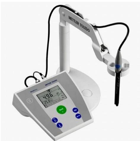
**Slika 7.** pH metar S20 SevenEasy Mettler Toledo
