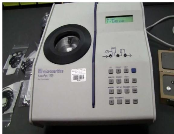
*Slika 14.* Micromeritics Accupyc 1330
