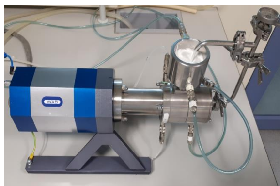
Slika 10. Mlin Dyno-mill Research Lab ( WAB, Švicarska )
