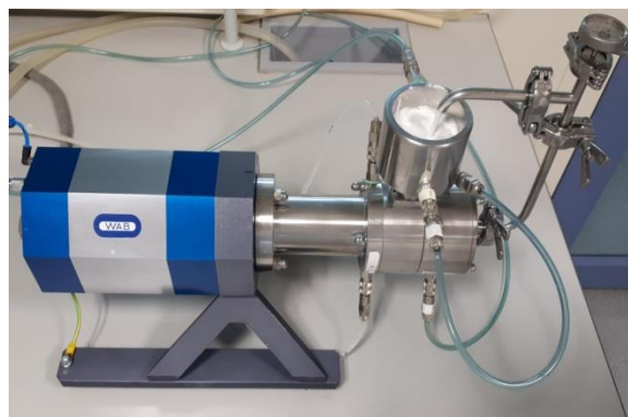
Slika 10. Mlin Dyno-mill Research Lab ( WAB, Švicarska )
