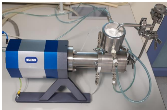
Slika 10. Mlin Dyno-mill Research Lab ( WAB, Švicarska )
