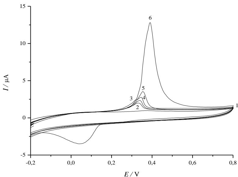
**Slika 22.** Ciklički voltamogrami dobiveni dodatkom  $50 \mu\text{L}$  vodljive tinte,  $w(\text{AgNP-PAA}) = 3,62\%$ , u  $10 \text{ mL}$  BR pufera raspona pH vrijednosti  $5,500 - 3,50$ , taloženo s  $0,01 \text{ M} \text{ H}_3\text{PO}_4$ .
