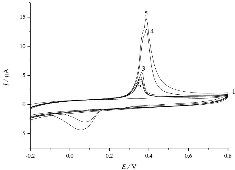
**Slika 30.** Ciklički voltamogrami dobiveni dodatkom  $50 \mu\text{L}$  vodljive tinte,  $w(\text{AgNP-PAA}) = 3,62\%$ , u  $10 \text{ mL}$  BR pufera raspona pH vrijednosti  $5,75 - 3,50$ , taloženo s  $0,01 \text{ M} \text{ H}_2\text{C}_2\text{O}_4$ .
