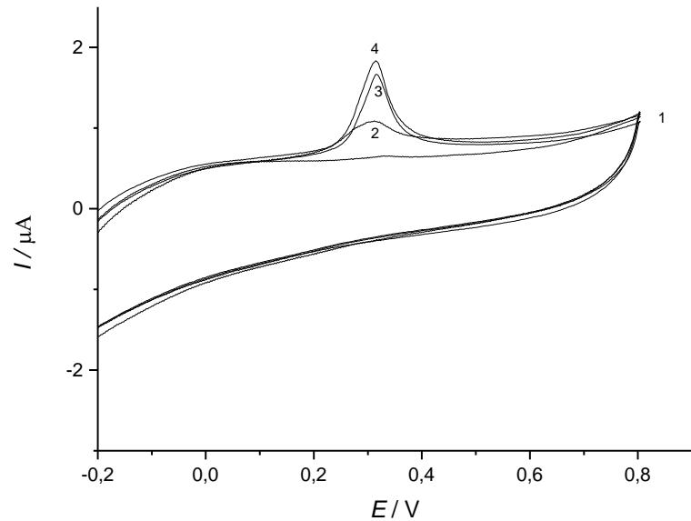
**Slika 54.** Ciklički voltamogrami dobiveni dodatkom  $50 \mu\text{L}$  vodljive tinte,  $w(\text{AgNP-PAA}) = 3,62\%$ , u  $10 \text{ mL}$  BR pufera raspona pH vrijednosti  $5,75 – 3,50$ . Taloženo s  $0,1 \text{ M}$   $\text{H}_2\text{SO}_4$ . **1** – osnovni elektrolit pH=  $5,75$ ; **4** – pH =  $5,75$ ; **3** – pH =  $5,50$ ; **2** – pH =  $5,00$ .
