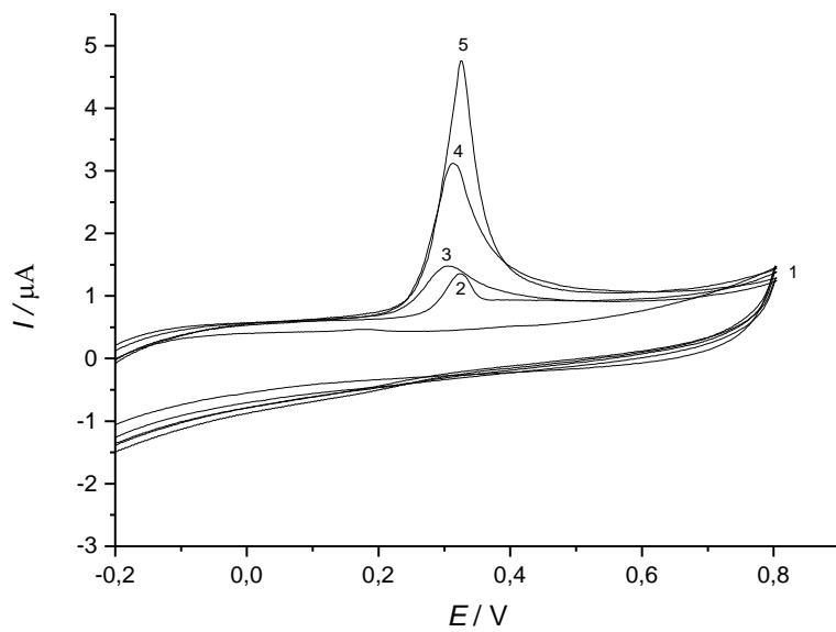
**Slika 53.** Ciklički voltamogrami dobiveni dodatkom  $50 \mu\text{L}$  AgNP-PAA tinte u  $10 \text{ mL}$  BR pufera u rasponu pH vrijednosti  $10,00 – 6,00$ . Taloženo s  $0,1 \text{ M}$   $\text{H}_2\text{SO}_4$ . **1** – osnovni elektrolit; **5** – pH =  $6,00$ ; **4** – pH =  $6,50$ ; **3** – pH =  $7,50$ ; **2** – pH =  $9,00$ .
