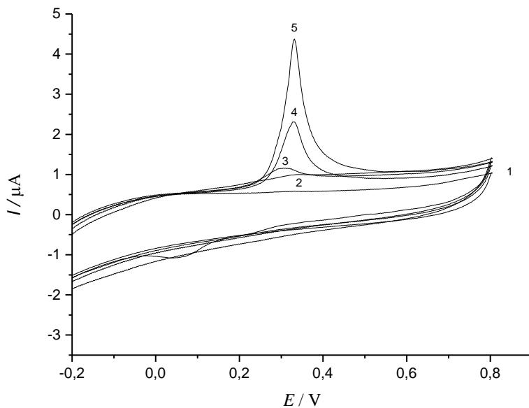
**Slika 46.** Ciklički voltamogrami dobiveni dodatkom  $50 \mu\text{L}$  vodljive tinte,  $w(\text{AgNP-PAA}) = 3,62\%$ , u  $10 \text{ mL}$  BR pufera raspona pH vrijednosti  $5,75 - 3,50$ . **1** – osnovni elektrolit; **5** – pH =  $5,75$ ; **4** – pH =  $5,50$ ; **3** – pH =  $5,00$ ; **2** – pH =  $3,50$ .
