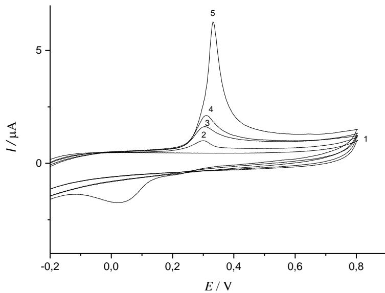
**Slika 45.** Ciklički voltamogrami dobiveni dodatkom  $50 \mu\text{L}$  vodljive tinte,  $w(\text{AgNP-PAA}) = 3,62\%$ , u  $10 \text{ mL}$  BR pufera u rasponu pH vrijednosti  $10,00 - 6,00$ . **1** – osnovni elektrolit bez dodatka AgNP pH =  $10,00$ ; **5** – pH =  $6,00$ ; **4** – pH =  $6,50$ ; **3** – pH =  $7,00$ ; **2** – pH =  $10,00$ .
