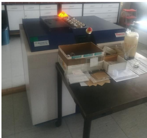
Slika 26. Valno-disperzivni X-ray spektrometar ARL ADVANT'X+ Sequential XRF, (Thermo)
