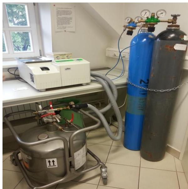
Slika 21. DSC instrument Mettler Toledo DSC 822<sup>e</sup>
