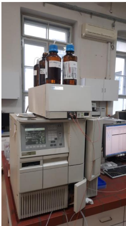
Figure 30. Waters 2795 Alliance HPLC system with 2996 PDA detector
