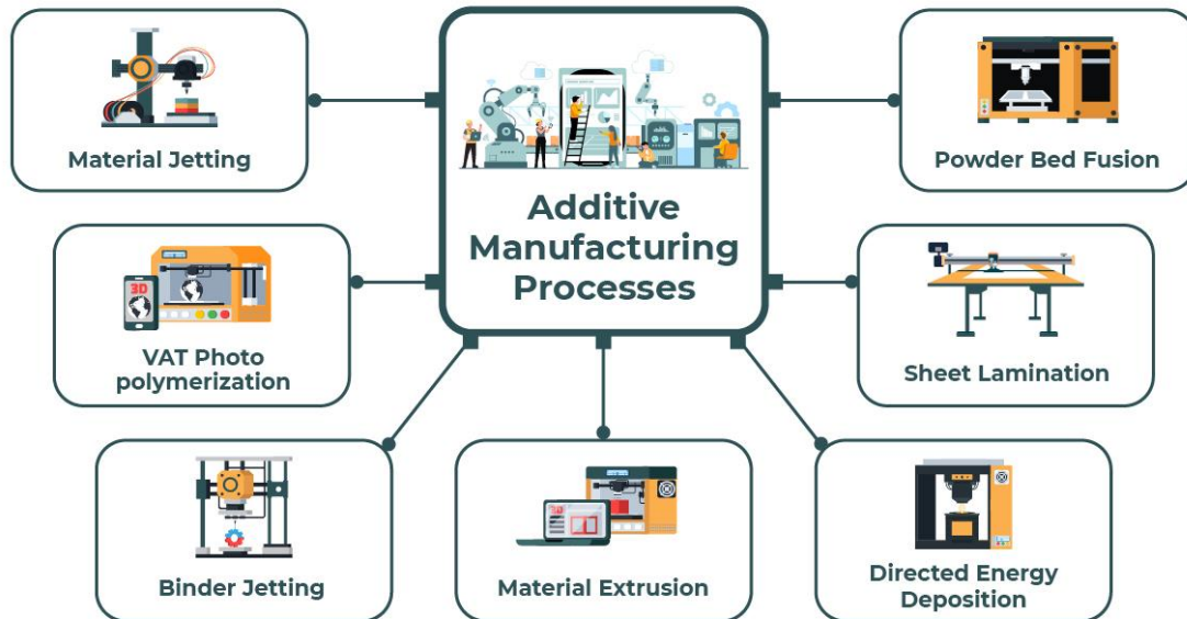
Figure 2.2. AM processes classified by Stucker et al. in the CRC Material Processing Handbook [5]
