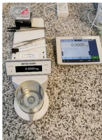
*Slika 6.* Mikrovaga Mettler Toledo XPR2U
