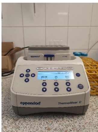
Slika 15. Termostatska tresilica Eppendorf ThermoMixer C .
