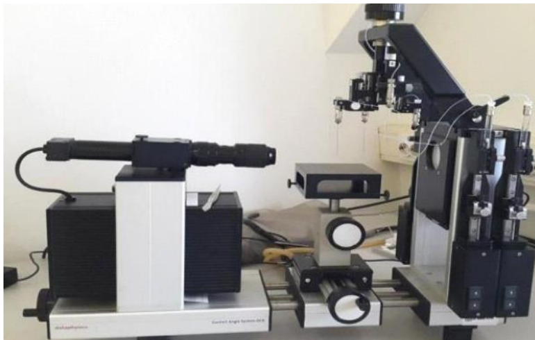
Slika 11. Goniometar DataPhysics OCA 20, Instruments GmbH
