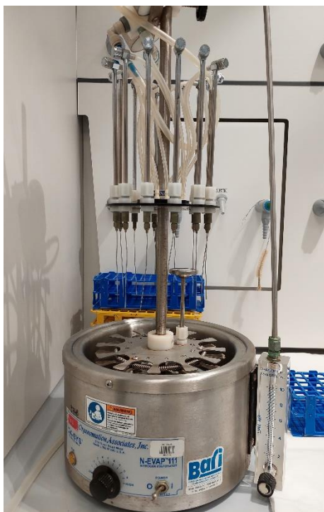
Slika 7. Uparivač u struji dušika Organomation Associates, USA
