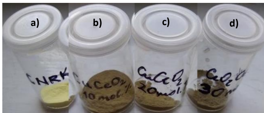
Slika 25. Promjena boje \text{Cu}:\text{CeO}_2 uzoraka; a) nanočestice \text{CeO}_2 , b) nanočestice 10 % \text{Cu}:\text{CeO}_2 , c) nanočestice 20 % \text{Cu}:\text{CeO}_2 i d) nanočestice 30 % \text{Cu}:\text{CeO}_2
