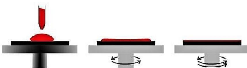
Figure 3. Different stages of spin coating [26].
