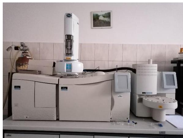
**Slika 4.** GC/MS instrument Clarus 500
