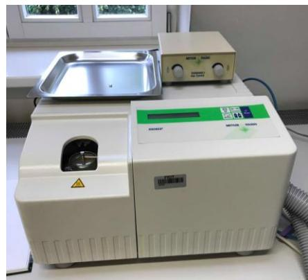
**Slika 22.** DSC analizator 822<sup>e</sup>, Mettler Toledo.
