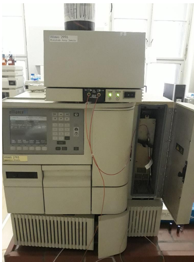
Slika 9. HPLC-PDA kromatograf Alliance 2795, Waters 2996
