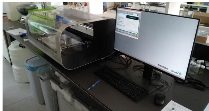
Slika 8. FUJIFILM Dimatix Materials Printer DMP-2850.
