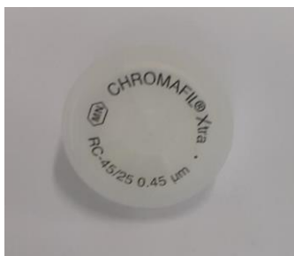
Slika 8. Filter CHROMAFIL® Xtra, RC-45/25 0.45 µm
