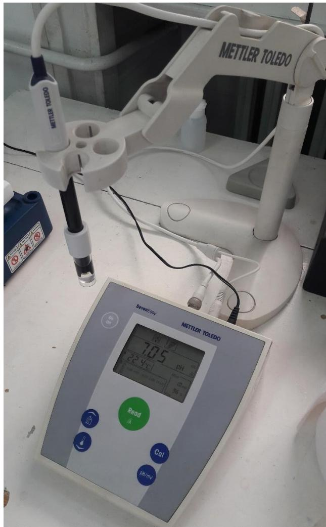
Slika 11. pH metar Mettler Toledo, SevenEasy
