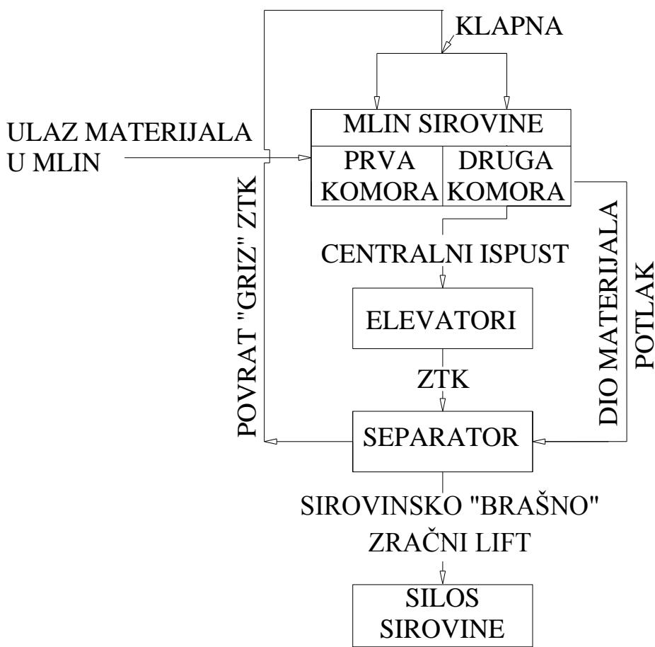
Slika 5. Blok shema mlin sirovine – silos sirovine
