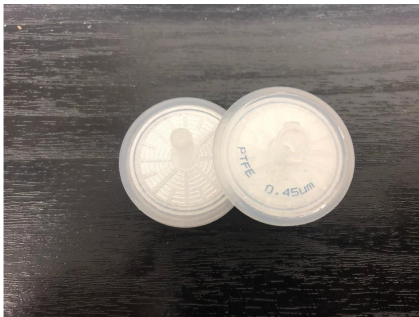
Slika 3.15. PTFE ( Polytetrafluoroethylene ) filteri
