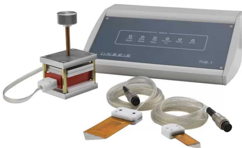
Slika 9. Transient Hot Bridge (THB) Thermal Conductivity Meter.
