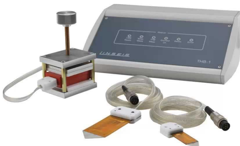
Slika 9. Transient Hot Bridge (THB) Thermal Conductivity Meter.
