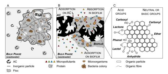
**Figure 3.4**. Schematic representation of a sludge floc in the bioreactor in the presence of AC (A); OMP removal mechanisms in an AC particle incorporated in the sludge floc (B); main functional groups on the surface of AC (C).
