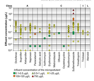
**Fig. 8.** Concentrations of micropollutants in the effluent of MBR + PAC for some classes of micropollutants. Data are provided with respect to the micropollutants concentration in the corresponding influent.
