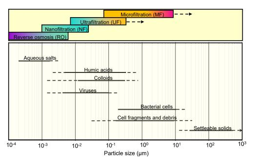
**Figure 1.2**. Size range of the constituents commonly found in wastewater and the operating size ranges for membrane technologies. Adapted from Metcalf and Eddy, (Metcalf & Eddy, 2014).
