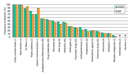
**Figure 5.7.** Frequency of detection (in percentage) of each OMP class in WWTP influent (INF) and hospital wastewater (HWW). In between brackets, the number of compounds for each class. Two classes, namely antihistamines and diuretics, were not detected in both HWW and INF (marked as \*).
