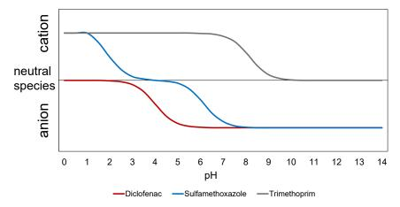
**Figure 6.4.** Changes in the ionization state of DCF, SMX and TMP as a function of the pH. J Chem for Office (20.11.0, ChemAxon, https://www.chemaxon.com) was used for calculating the physicochemical properties and ionization state.
