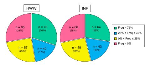
**Figure 5.6.** Frequency of detection (Freq) of the 232 OMPs analysed in the hospital wastewater (HWW) and WWTP influent (INF), categorized into four groups: Freq > 75% (green); 25% < Freq ≤ 75% (blue); 0% < Freq ≤ 25% (yellow) and Freq = 0% (pink). *n* indicates the number of compounds for each group, with the percentage they represent in between brackets.
