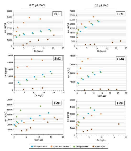
**Figure 6.10.** Experimental equilibrium adsorption capacity of DCF, SMX and TMP at two different PAC concentrations (0.25 and 0.5 g/L) in ultra-pure water, humic acid solution, MBR permeate and mixed liquor from a WWTP.
