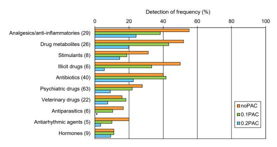
**Figure 5.11**. Detection of frequency (%) of the main OMP classes (number of OMPs > 5) in the MBR permeate (*MBRperm*) for MBR (*noPAC*), MBR+0.1 g/L PAC (*0.1PAC*) and MBR+0.2 g/LPAC (*0.2PAC*) treatments. In the case of the antiparasitics class, no compound was detected during *0.2PAC* treatment (marked as \*).
