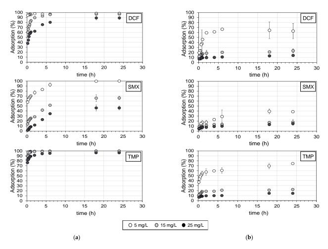
**Figure 2.** Kinetics of adsorption of DCF, SMX and TMP at three different concentrations in Milli-Q water with (a) 1 g/L of PAC and (b) 0.1 g/L of PAC at different contact times (10 min–24 h). Error bars indicate the standard deviation.
