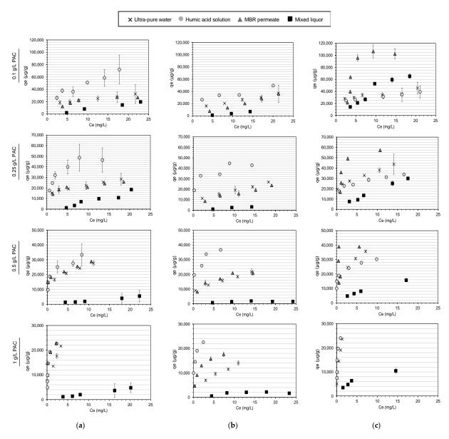
**Figure 4.** Experimental equilibrium adsorption capacity of (a) DCF, (b) SMX and (c) TMP at four different PAC concentrations (0.1, 0.25, 0.5 and 1 g/L) in ultra-pure water  $(\times)$ , humic acid solution  $(\bigcirc)$ , MBR permeate ( $\blacktriangle$ ) and mixed liquor from a WWTP ( $\blacksquare$ ). Error bars indicate the standard deviation.
