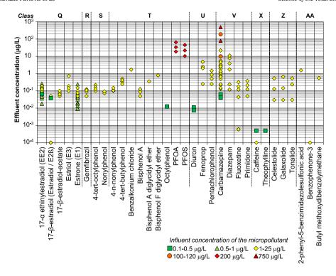
**Fig. 9.** Concentration in the effluent of MBR + PAC for micropollutants belonging to the other classes included in the review. Data from: Alvarino et al. (2016, 2017); Asif et al. (2020); Echevarría et al. (2019); Li et al. (2011); Nguyen et al. (2013a); Remy et al. (2012); Serrano et al. (2011); and Yu et al. (2014).
