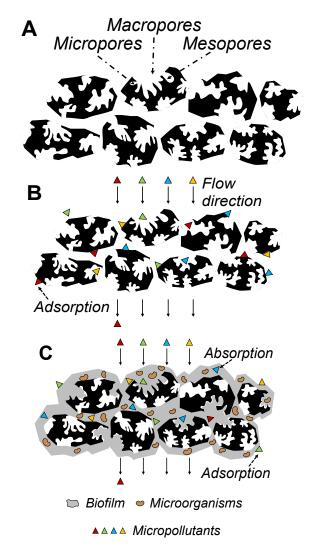
**Figure 3.3.** Schematic representation of (A) the structure of activated carbon; (B) adsorption of micropollutants on the surface of the AC; (C) BAC, with micropollutants absorbed and adsorbed on its surface.
