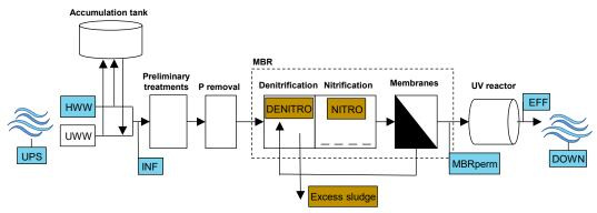
**Figure 5.2.** Sampling points of wastewater (in blue) and mixed liquor/sludge (brown). Wastewater samples were taken in six sampling points: hospital wastewater (HWW); WWTP influent (INF); MBR permeate (MBRperm), final effluent (EFF) and in the irrigation ditch, both upstream (UPS) and downstream (DOWN) the WWTP.
