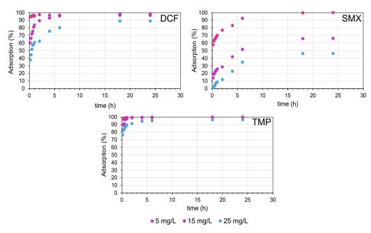
**Figure 6.5**. Kinetics of adsorption of DCF, SMX and TMP at three different concentrations (5, 15 and 25 mg/L) in Milli-Q water with 1 g/L of PAC at different contact times (10 min - 24 h).
