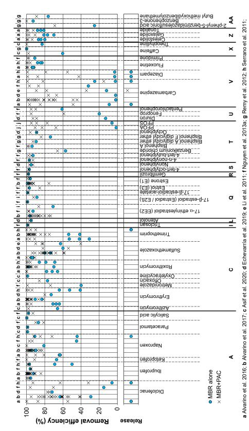
Figure 3.5. Comparison among removal efficiencies achieved in MBR alone and MBR coupled with PAC. While lower case letters refer to the referenced studies, capital letters group the compounds by class according to Table 3.1. The separate grid at the bottom of the graphic indicates the release of the OMP, that is, i Yang et al. 2012; j Yu et al. 2014
