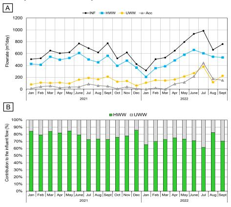
**Figure 5.5**. Description of the flowrate entering the WWTP: a) Flowrate (m³/day) of the urban wastewater (UWW), hospital wastewater (HWW), and accumulation tank (Acc) entering the WWTP (INF) (sum of UWW and HWW). Note that the Acc flowrate represents a mixture of HWW and UWW entering the WWTP in case strong rainy events take place. b) Ratio (%) of HWW and UWW contributing to the WWTP influent flow.
