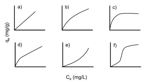
**Figure 1.8**. Representation of different isotherm types.  $C_e$  is the equilibrium concentration of the adsorbate in the liquid phase and  $q_e$  is the amount of adsorbate per mass unit of adsorbent. Adapted from Schwarzenbach et al., (2002).
