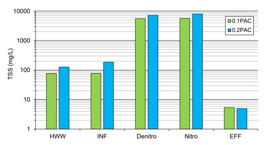
**Figure 5.3**. Concentration of total suspended solids (TSS) in HWW, INF and EFF, together with the DENITRO and NITRO MBR compartments. Green and blue colours correspond to the concentrations of *0.1PAC* and *0.2PAC* experimental campaigns, respectively.
