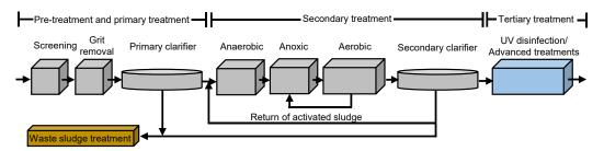
Figure 1.1. Diagram of conventional WWTP.
