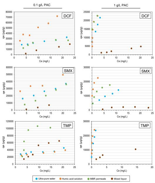
**Figure 6.9**. Experimental equilibrium adsorption capacity of DCF, SMX and TMP at two different PAC concentrations (0.1 and 1 g/L) in ultra-pure water, humic acid solution, MBR permeate and mixed liquor from a WWTP.
