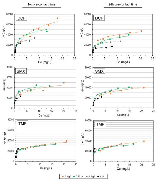
**Figure 6.11.** Experimental adsorption capacity of PAC at four concentrations (0.1, 0.25, 0.5 and 1 g/L) for individual OMPs (DCF, SMX and TMP) in a humic acid (HA) solution. In the left, OMPs and PAC were added at the same time to the HA solution (no pre-contact time). In the right, each OMP was added to the HA solution 24 h before the PAC addition (24 h pre-contact time).
