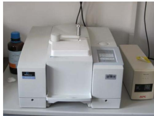
**Slika 14.** FTIR spektrometar, Perkin Elmer Spectrum One Spectrometer s ATR komorom
