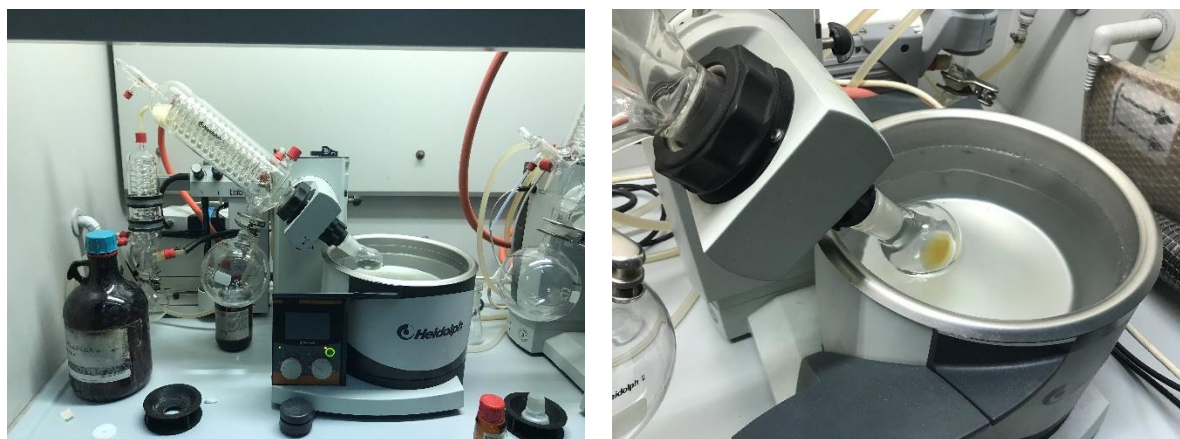
Figure 21 Removal of EtOAc under reduced pressure (Heidolph, Germany) to yield thick (viscous) CDH product.
