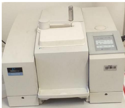
Slika 11. FTIR spektrometar Perkin-Elmer model Spectrum One.
