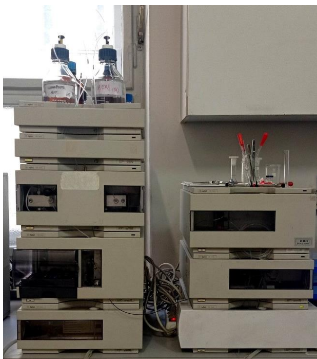
Slika 22. HPLC Agilent Series 1100 s DAD detektorom
