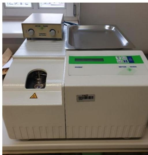
Slika 22. DSC instrument, Mettler Toledo DSC 822<sup>e</sup>
