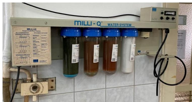
*Slika 24.* Milli-Q Reagent Grade Water System, Millipore Corporation
