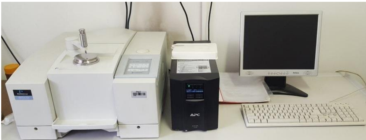
Slika 34. FTIR-ATR spektrometar, Perkin Elmer Spectrum One Spectrometer.
