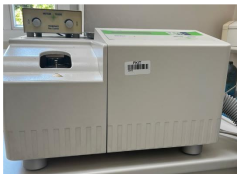
Slika 14. DSC instrument Mettler Toledo DSC 82
