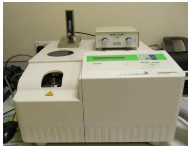
*Slika 22.* Mettler Toledo DSC 823eT kalorimetar
