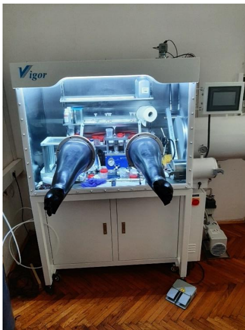
Slika 3.3. Komora s atmosferom argona – „ Glove Box “ SG1200/750TS (Vigor Technologies, Kina)
