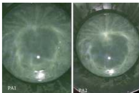
Figure 49: Samples PA1 and PA2 in the can with defects such as flocculation, lack of stabilization of pigments in the coating vehicle and blushing
