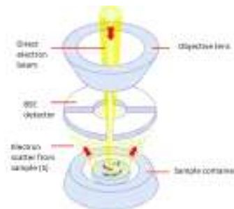
Figure 44: The location of the BSE detector
