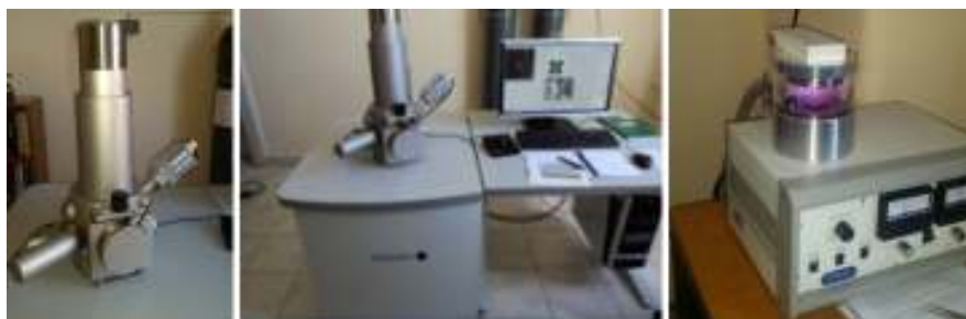
Figure 42: Scanning Electron Microscope (SEM)
