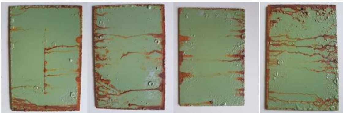
Figure 55: The sample PA6, the results of testing in a salt spray cabinet
