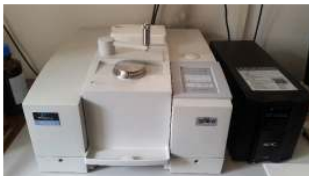
Figure 38: Fourier-transform infrared spectroscopy apparatus (FTIR)
