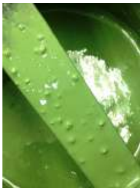
Figure 53: Incompatibility in the sample PA6
