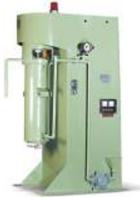
Figure 29: The laboratory pearl mill PS-C, 3.5 liters, variable rotational speed
