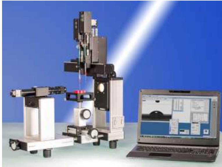
Figure 46: Goniometer DataPhysics OCA 20, Instrument for measuring the contact angle
