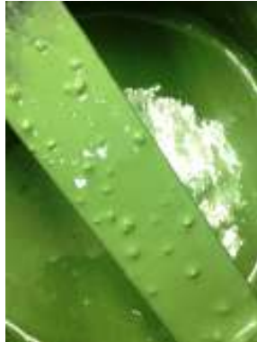
Figure 53: Incompatibility in the sample PA6
