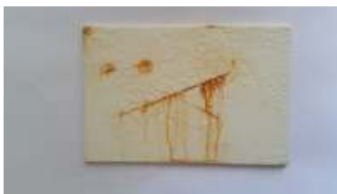
Figure 58: PA7-2 after 1000 h under the salt spray test before adding more adhesion promoter and surface agent
