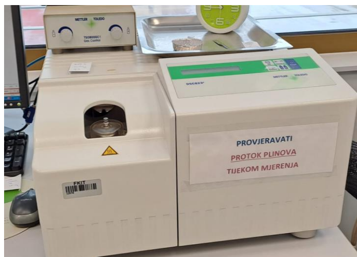
Slika 23. DSC instrument Mettler Toledo 823 e
