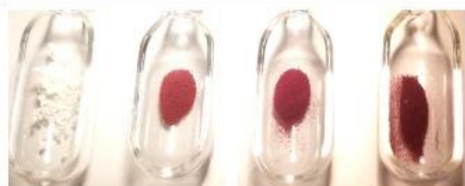
Figure 1. Different concentrations of C_{60} in mechanochemically prepared C_{60} @ZIF-8. From left to right: 0, 30, 60, and 100% C_{60} @ZIF-8, respectively.
