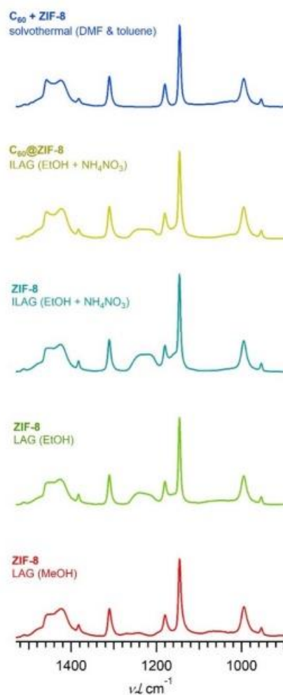
Figure S9. Comparison of the ZIF-8 samples prepared by different methods. The 1280-1200 \text{cm}^{-1} feature is present exclusively when EtOH was used in the synthetic process.
