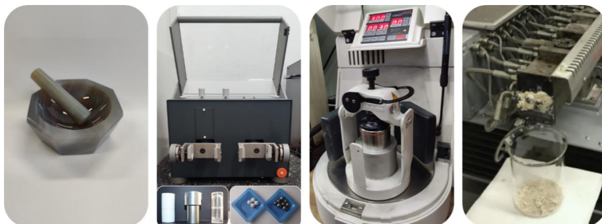
Figure 1. Standard equipment used for mechanochemical reactions. Left to right: mortar and pestle; mixer mill with milling vessels (Teflon, stainless steel, PMMA) and balls ( \text{ZrO}_2 , stainless steel); planetary mill with stainless steel milling vessel; twin-screw extruder.
