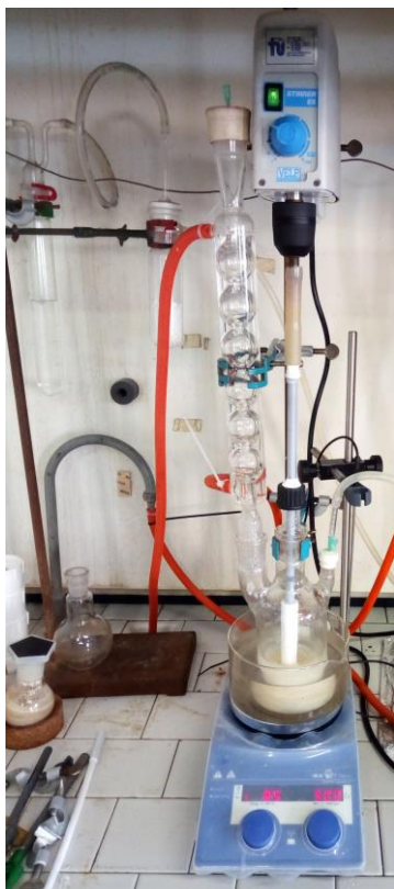
Figure 27. Suspension polymerization reactor used in laboratory
