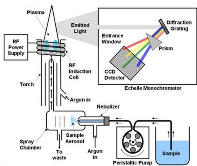
Fig. 2.7.1. Working principle of ICP- AES method <sup>42</sup>
