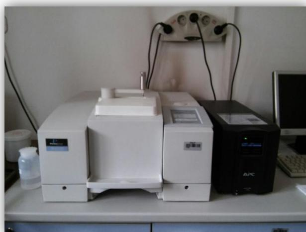
**Slika 18.** FT-IR spektrometar, Perkin Elmer Spectrum One Spectrometer
