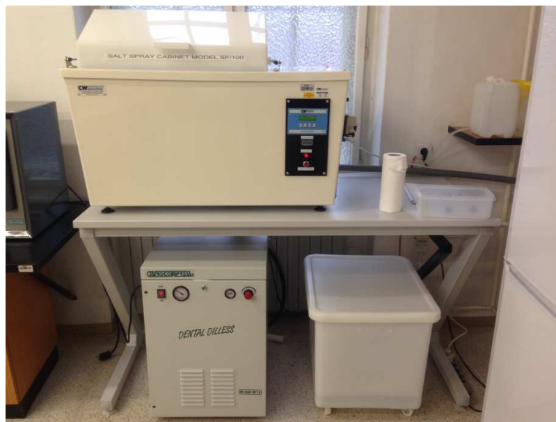
Slika 4. Slana komora (CW specialist equipment model SF/100)
