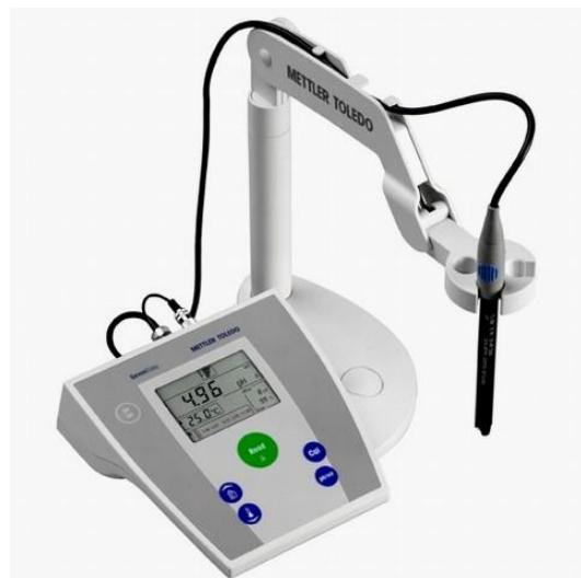
**Slika 11.** pH metar Mettler Toledo S20 SevenEasy
