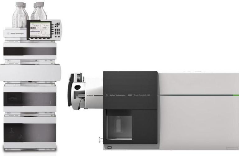
**Slika 12.** UHPLC Agilent Series 1290 i Agilent 6490 Triple Quad MS
