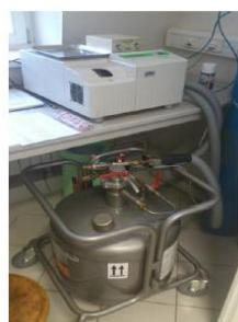
**Slika 15.** DSC analizator Mettler Toledo 822<sup>e</sup>
