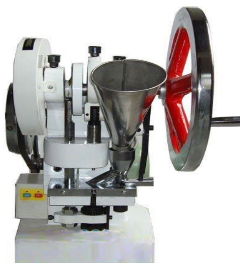
Slika 11. Tabletirka TDP-5T (Zhejiang wisely machinery co. Ltd, Kina)
