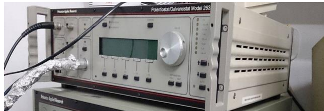
Slika 3.8. Potenciostat EG&G Princeton Applied Research, model 263A
