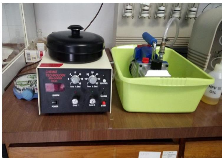
**Slika 12.** *Spin coater*, Chemat Technology.
